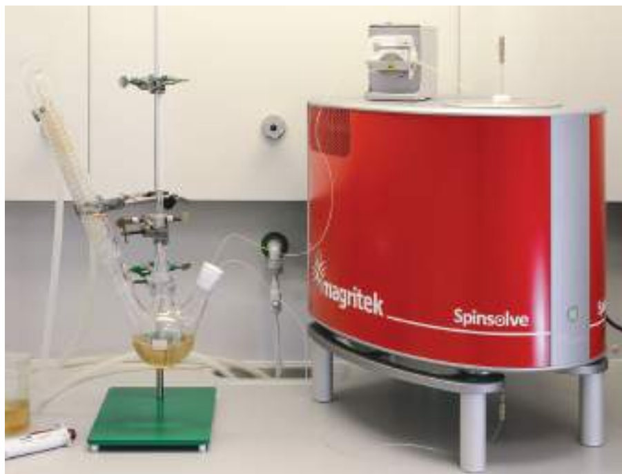
Reaction monitoring with the Spinsolve® Benchtop NMR spectrometer and the glass flow cell.
